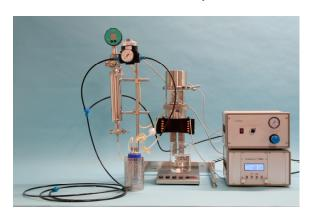
During the work with very low pressure the drops wond be produced, but there will be a laminar jet smaller than the nozzle applied. If the vibration would be superimposed the even sized beads down to half the size of the applied nozzle could be produced.
